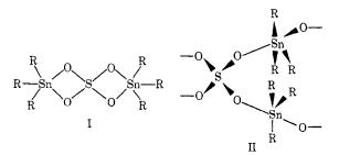
metry for the XO<sub>4</sub> groups, and the tin-carbon stretching frequency regions show only  $\nu(\text{Sn-C}_3)_{asym}$ . For  $[(\text{CH}_3)_8\text{Sn}]_2\text{SO}_4$ , the Raman spectrum<sup>5</sup> shows only  $\nu(\text{Sn-C}_3)_{sym}$ . These results clearly suggest a planar (CH<sub>3</sub>)<sub>3</sub>Sn moiety and are thus consistent with structure II and inconsistent with I.<sup>2-4</sup>
